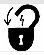
Never attempt to service a unit until a qualified electrician has opened and locked out the main disconnect using OSHA 1910.147 standards.
